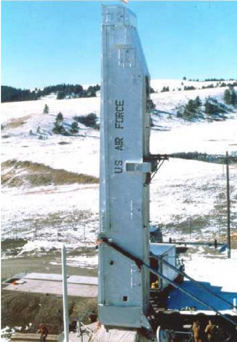
**Maintenance is performed in some of the most austere weather conditions around. Here a transporter erector inserts a Minuteman ICBM into its underground silo.**
