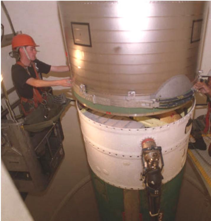
**A credible nuclear deterrent is dependent in part on a skilled maintenance force. Here a maintenance team installs a reentry system on top of a Minuteman III.**
